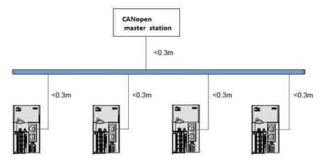
If you use the topological interface in the figure above, pay attention that the length of each branch is less than 0.3m. Whether it will cause reflections and cause communication problems.
