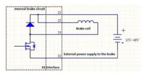
• The maximum output current of the brake is 2.2A, with internal current limiting protection.
